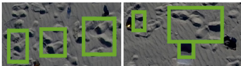
Fig. 8. Examples of shadows in the proximity of footprints (left image) and of items of AMD (right image), that are mistaken as AMD by the software, representing pitfalls for the algorithm in its present version.
