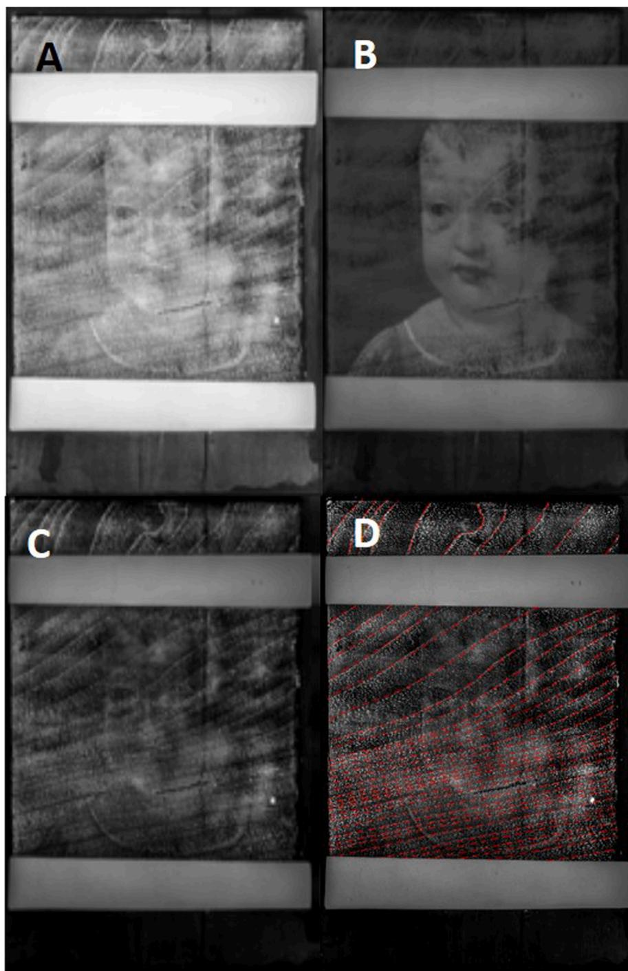
**Fig. 1.** A) RX image; B) RX elaborated image highlighting the radiopaque layer of imprimatura; C) RX elaborated image D) eye-guide for the original wood panel.
