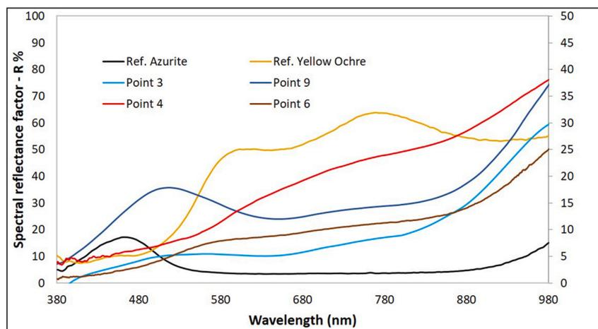
Fig. 14. Reflectance spectra for the Virgin and Child pane by an unknown painter (for the point location, see Fig. 1S).
