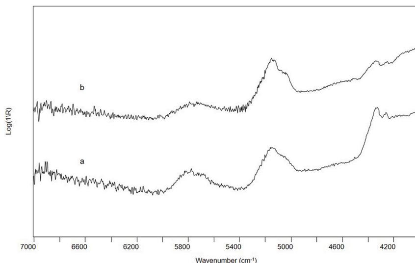
Fig. 2. FT-NIR reflection spectra of (a) area 2 and (b) area 3 of the painting “Virgin and Child” by G. Boltraffio.
